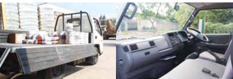
Its unique selling point, though, is a gross vehicle mass (GVM) of 3 495 kg, a tare mass of 1 865 kg, and a payload of 1 630 kg. When these figures are added together it means that the Carrying can be driven by anybody with a basic code 8 driving licence.
